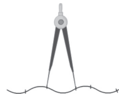
Measuring the length of a curved line with the help of a divider
